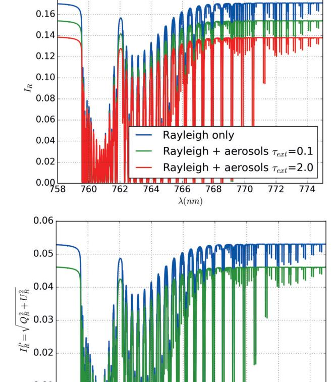
TOA reflectance for an atmosphere with desert aerosols over glitter for the full TANSO-FTS1 range with a resolution of  $10^{-2}$  cm<sup>-1</sup> (SZA=30°,  $VZA=20^{\circ}$ ,  $RAA=0^{\circ}$ ,  $N_{WVI}=27137$ ).
