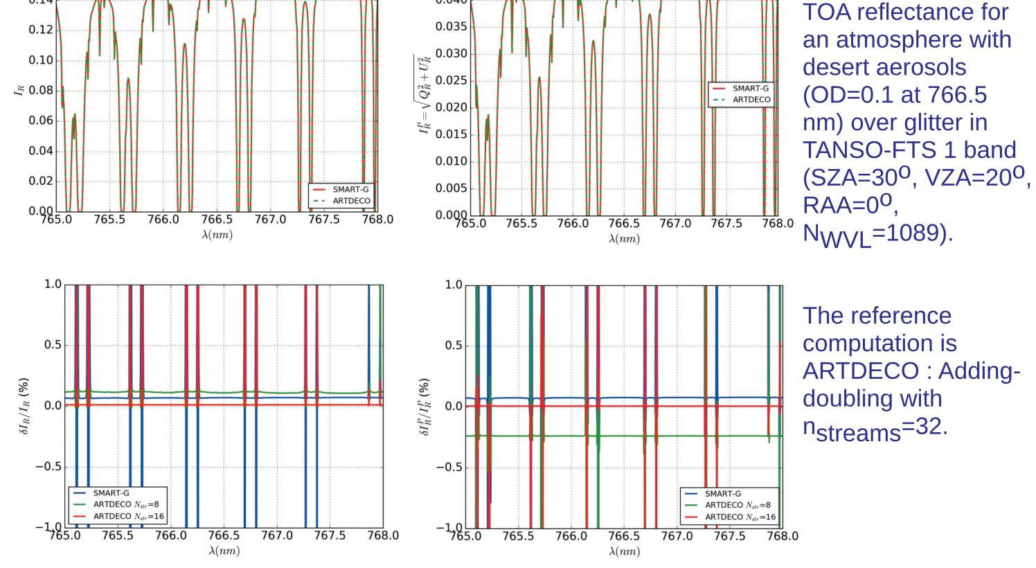
SMART-G results have a relative error < 0.1%. SMART-G computing time is  $\sim 2.70$ s for  $10^6$ photons. ARTDECO computing time is  $\sim$ 620s with  $n_{streams}$ =16 on a single CPU.
