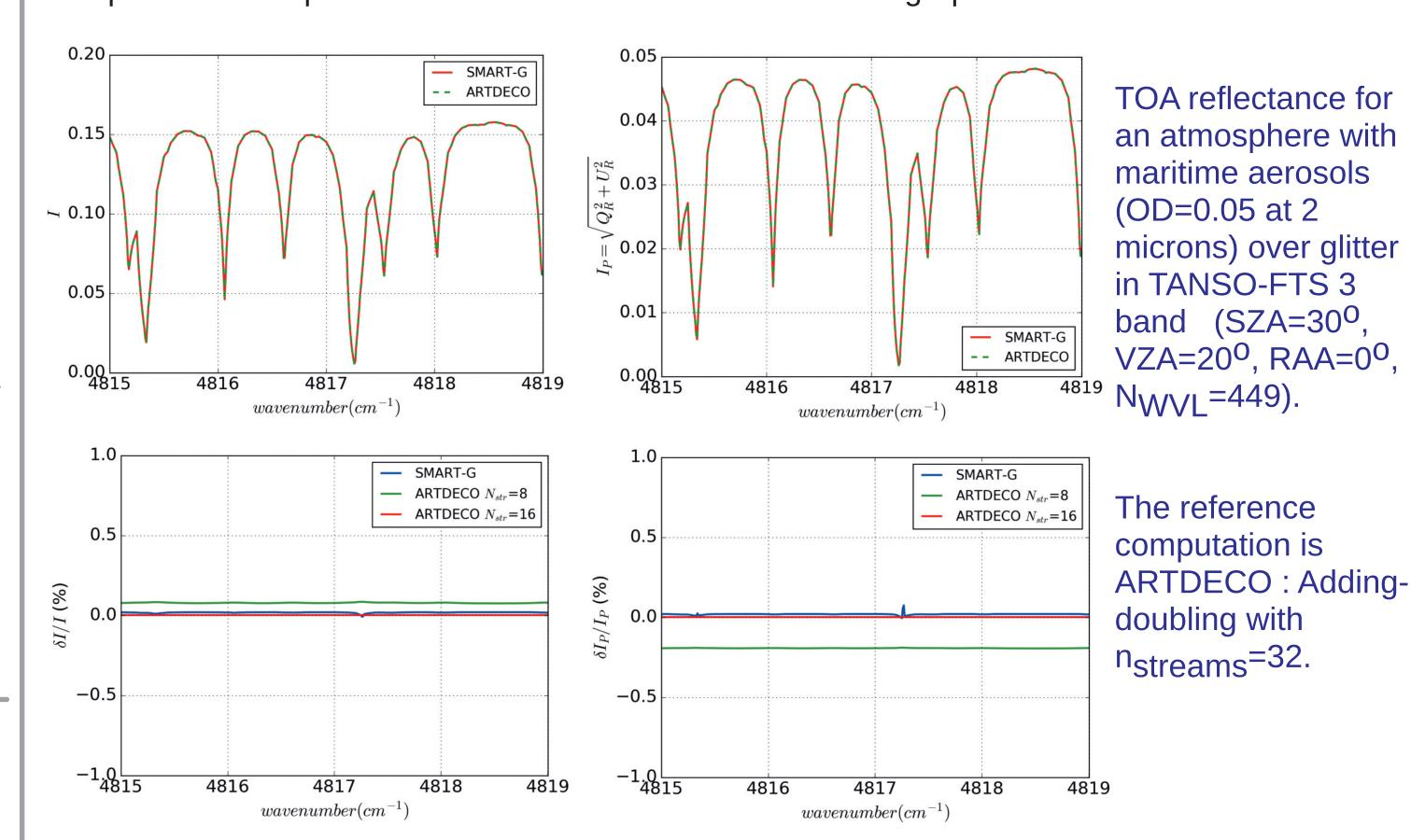
SMART-G results have a relative error < 0.1%. SMART-G computing time is  $\sim$ 1.2s for  $10^6$ photons. ARTDECO computing time is  $\sim$ 210s with  $n_{streams}$ =16 on a single CPU. Same computation with MYSTIC/ALIS on a single CPU is ~145s (Emde et al., 2011).
