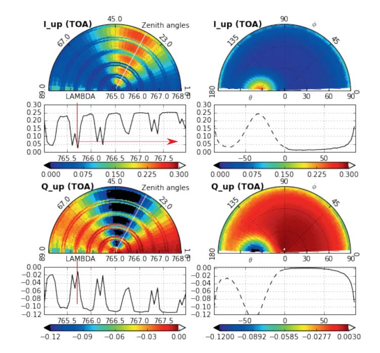
$\blacktriangleleft$  Part of  $O_2$  A bands. I and Q spectra are computed at TOA with a clear sky over the sun glint (wind speed 5 *m/s). The sun zenith angle is* 30 deg. The observation geometry is that of the glitter's maximum reflectance. The absorption coefficient are obtained from the REPTRAN parametrization (Gasteiger et al. 2014) with channels of 1 cm<sup>-1</sup> width
