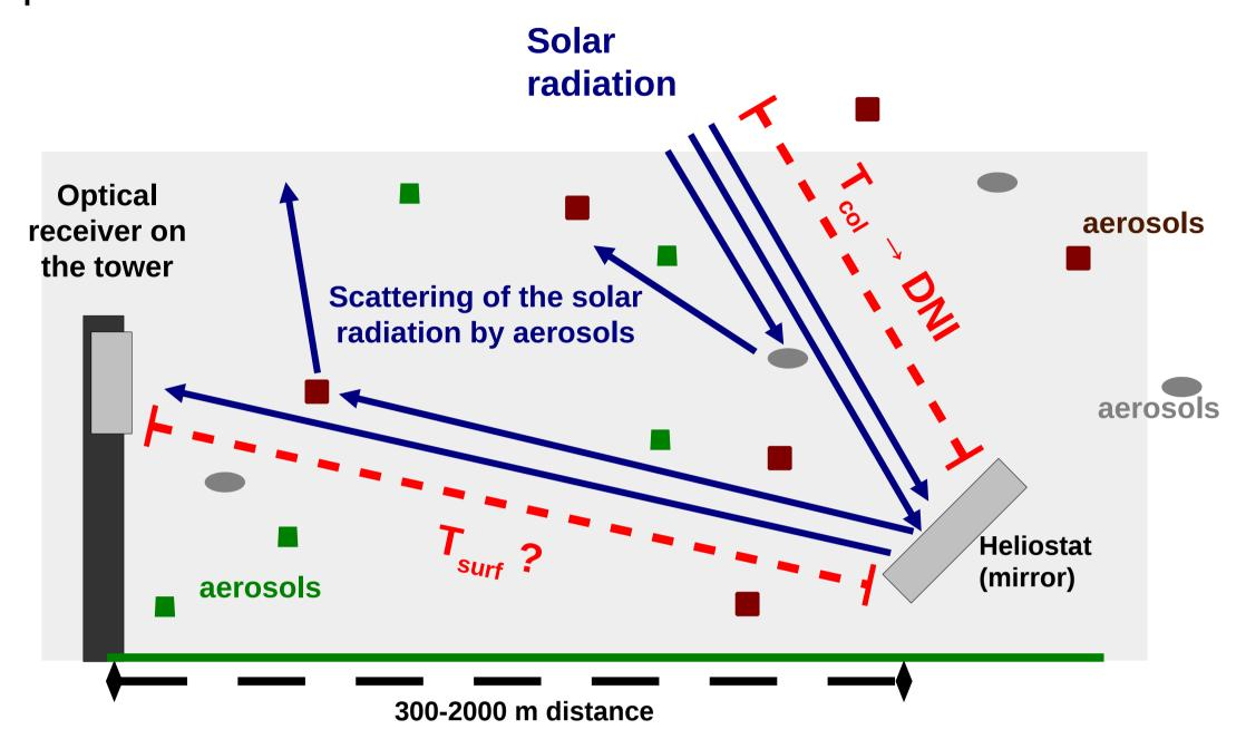
Figure 1. Schematic view of the two optical pathways in a tower STE plant, and the scattering effect by aerosols.
