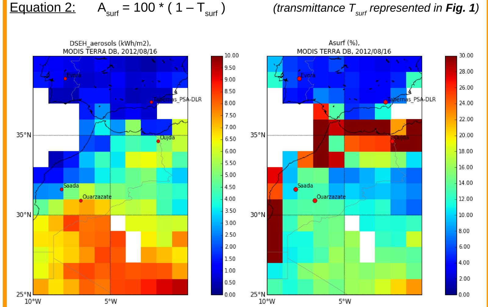
**Figure 2.** Solar resource parameters computed with MODIS AOT (Collection 6, Level 3, Deep Blue algorithm), MODIS water vapour content, MODIS ozone content, ECMWF ERAinterim BLH, on 16 August 2012 at around noon. ΔSEH<sub>aerosol</sub> (kWh/m²) is showed on the left, and A<sub>surf</sub> (%) on the right. No clouds are considered in the coloured pixels, while white pixels indicate cloud presence. AERONET stations are indicated.
