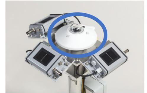
Fig. 2. PV-Live measurement station with a horizontally mounted pyranometer and three silicon reference cells with tilt angles of 25°. The stations are installed with the orientation of the Si Sensors towards east, south, and west.
