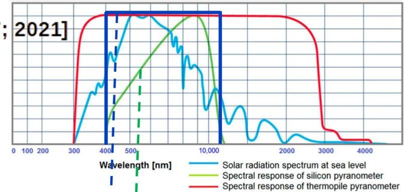
Figure 3. Spectral response curves of silicon, thermopile pyranometers, and solar spectrum at sea level [20].
