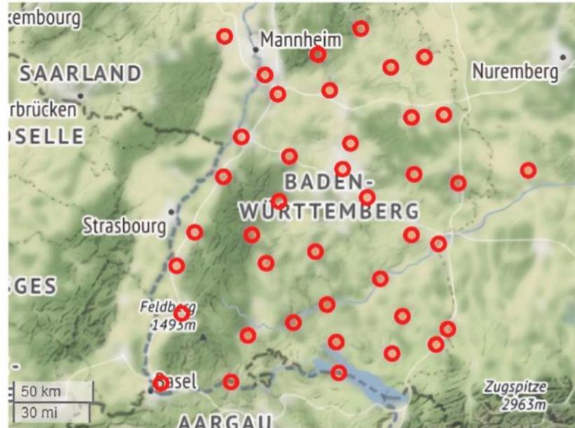
Fig. 1. The PV-Live network consists of 40 measurement stations distributed over the control area of TransnetBW, corresponding widely to the state of Baden-Württemberg in Germany, which covers an area of about 35.751 km<sup>2</sup> (Map tiles by Stamen Design (<https://stamen.com>), under CC BY 3.0. Data by OpenStreetMap, under ODbL (<https://www.openstreetmap.org/copyright>)).
