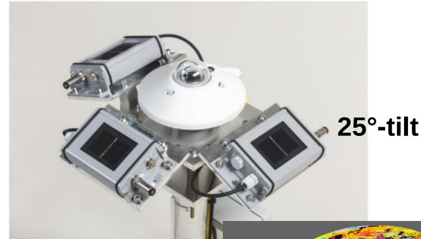
Fig. 2. PV-Live measurement station with a horizontal orientation of the three silicon reference cells with tilt angles of 25°. The orientation of the Si Sensors towards east, south,
